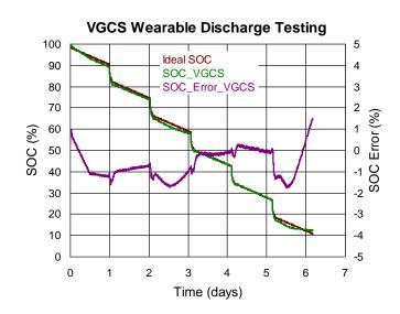
Figure 7. Performance of Capacity Estimation for Wearable Device with 7-Days Usage
