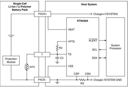
Figure 6. <u>RT9426A</u> Simplified Application Circuit
