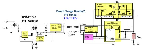
Figure 39. Structure of High Power Charging System
