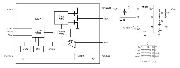
Figure 17. RT4813 Block Diagram, Simplified Circuit and Package
