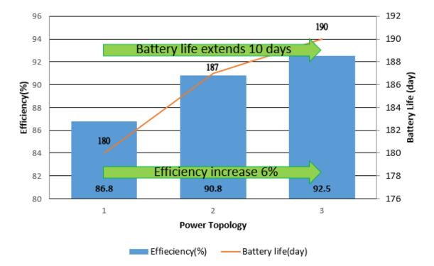
Figure 26. Battery Run Time Comparison between Different Power Topologies
