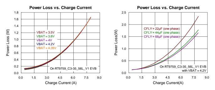
Figure 42. RT9759 Power Loss vs. Charge Current
