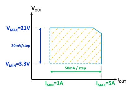
Figure 40. Programmable Power Supply (PPS) V/I Range
