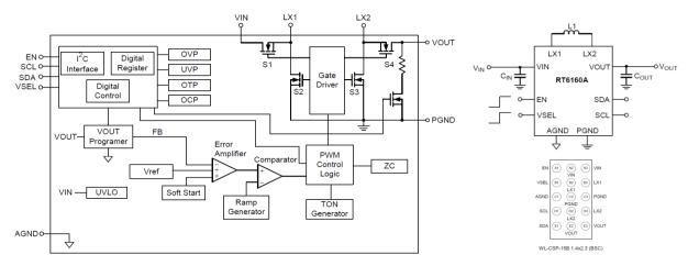
Figure 20. RT6160A Block Diagram, Simplified Circuit and Package
