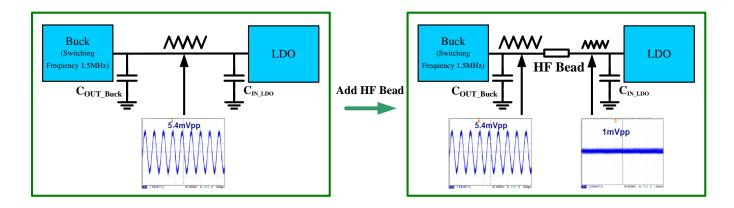
Figure 35. HF Bead Filter out HF Ripple
