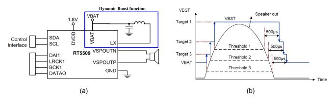
Figure 36. (a) Simplified Circuit of RT5509 (b) Class-G Boost Converter Behavior of RT5509
