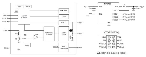
Figure 18. RT5707 Block Diagram, Simplified Circuit and Package
