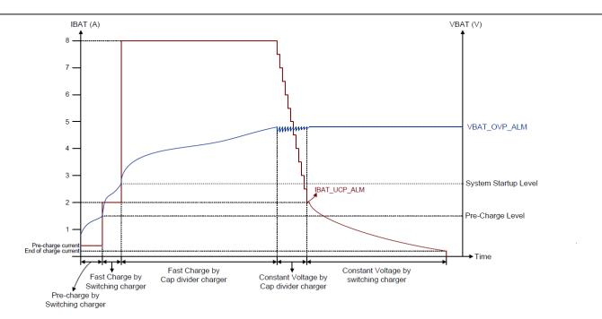
Figure 44. Charge Flow with Cap Divider Charger and Switching Charger
