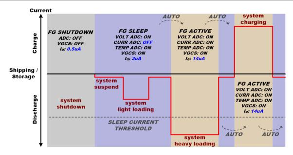
Figure 9. RT9426A Power Mode vs. System Loading
