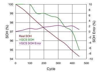
Figure 14. FCC Performance of 450 Cycles Usage
