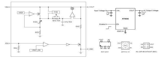
Figure 21. RT9086 Block Diagram, Simplified Circuit and Package
