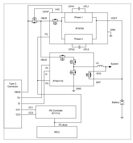
Figure 43. Simplified Charge System for Doorbell Power System
