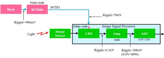
Figure 33. Power Requirement Deduction with RT9086 for AVDD
