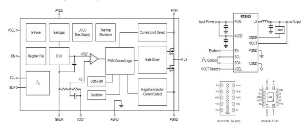
Figure 22. RT8092 Block Diagram, Simplified Circuit and Package
