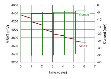
Figure 8. Battery Voltage & Current Profile of Wearable Device with 7-Days Usage
