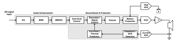
Figure 37. Speaker Protection Path of RT5509
